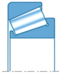
Gambar 4 Bearing NTN 4T 32203R
