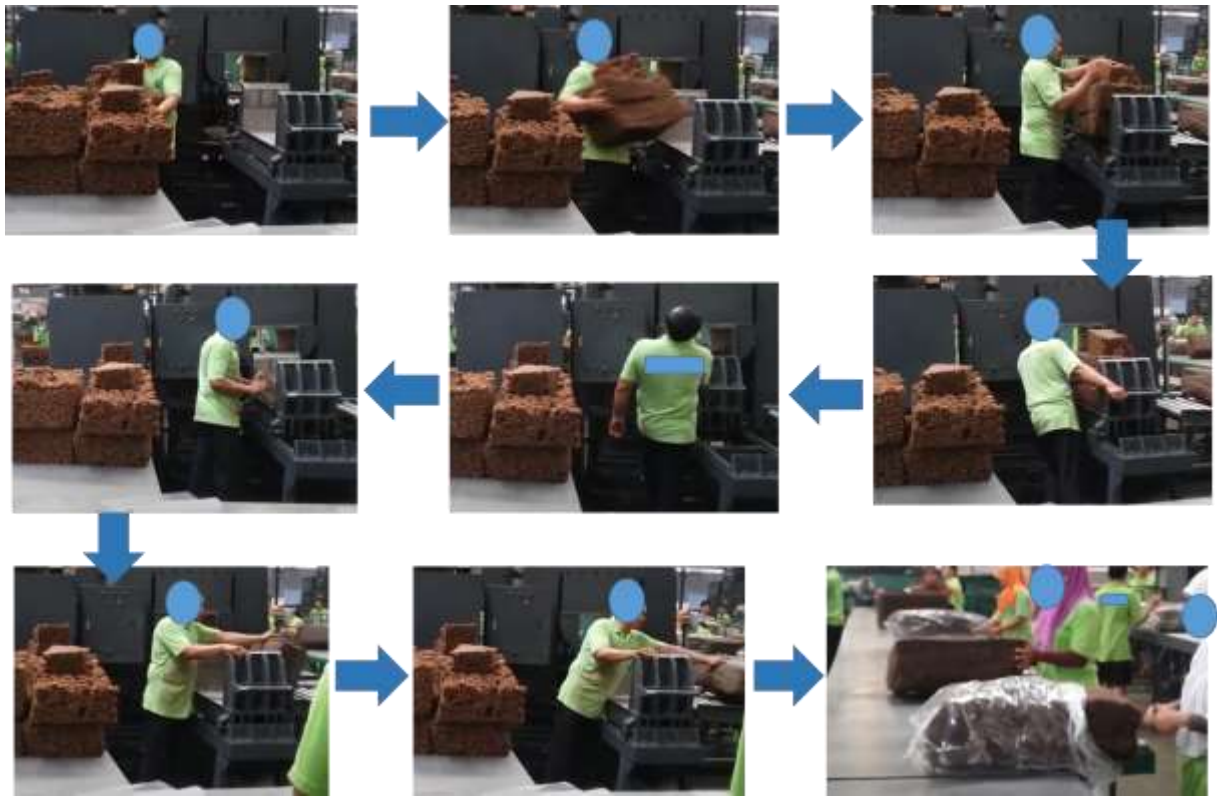
Gambar 2. Proses pengemasan crumb rubber (bandela)
