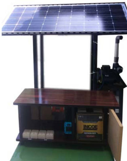
Gambar 2.2 Perancangan Solar Water Pump System
